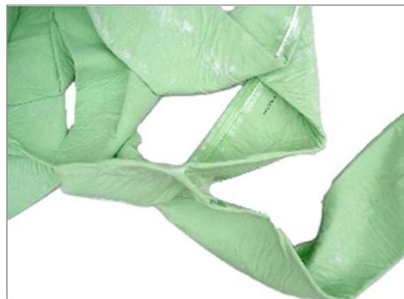
Flexible liner with “T” configuration
